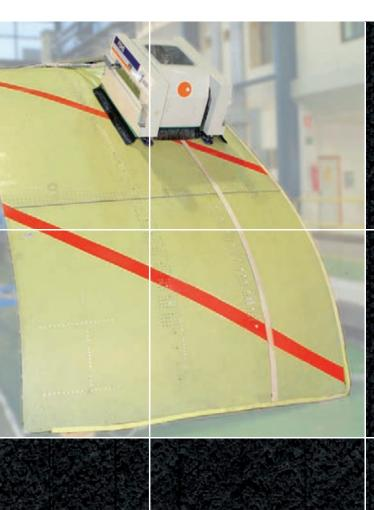
A 5 minutes set up on place by 2 operators is enough to be FLEXIBLE DRILLING HEAD (FDH) 5 Axis Drilling Crawler Robot is a portable and autonomous drilling and riveting standalone robot.
